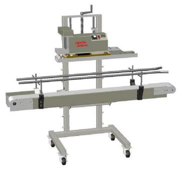
The SS1500-SSC545 **Sealer and Conveyor** is a workhorse when **Bag Packaging** products from the hardware industry to spices and sauces along with many other industries; these machines work very well with filling and assembly lines. They are perhaps the best solution for your **heavier heat sealing** applications that <u>do not</u> require trimming above the seal.
