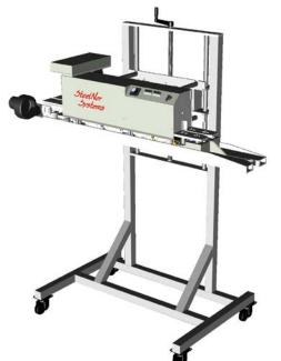
The **SS2525PTHD Sealer** is designed for **Large Bag Packaged** products used in the pet food industry; these machines work very well with filling and bag/sack placing lines and can be used with existing conveyors. They are perhaps the best solution for your **Heavy Duty Seal and Trim** applications, including heavy laminate materials.
